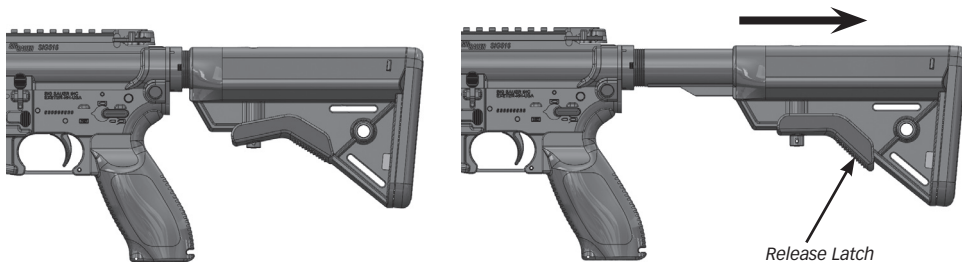
BUTT STOCK COLLAPSED AND FULLY EXTENDED
