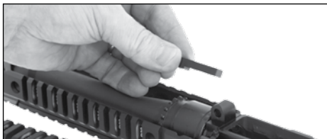
FIG 35 REMOVAL OF THE QUAD KEY FROM BARREL NUT
