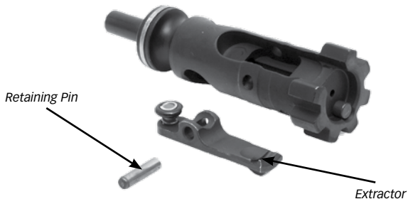
FIG 29 BOLT WITH EXTRACTOR REMOVED
