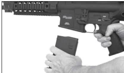
FIG 24 MAGAZINE BEING INSERTED
