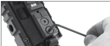
FIG 32 REMOVAL OF CLAMP SCREWS AND CLAMP
