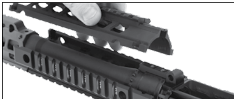
FIG 34 REMOVAL OF THE LOWER RAIL SECTION
