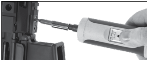
FIG 52 TIGHTENING OF RAIL CLAMP SCREWS
