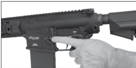
FIG 25 MAG CATCH BEING DEPRESSED LEFT AND RIGHT SIDE
