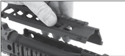
FIG 50 RE-INSTALLATION OF LOWER RAIL SECTION
